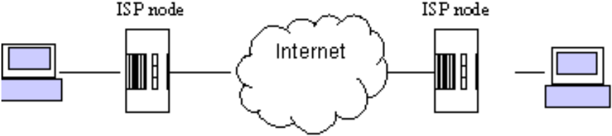
Fig 7: PC to PC communication for Internet telephony
