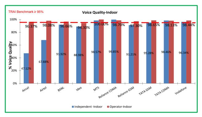
In indoor locations, Idea failed to meet the benchmark in both the drive tests.
