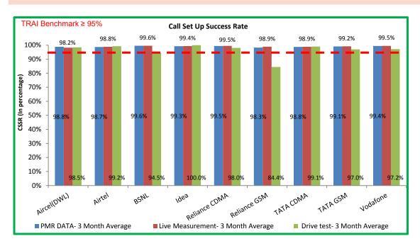
All the operators are meeting the benchmark across Monthly PMR, Live measurement and Drive Test. There is no significant difference for CSSR found except for Reliance GSM which had a lower CSSR for the drive test
